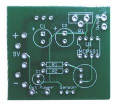
The Op-Amp circuit is designed to use a variety of resistive sensors and output a 0-5V DC.
