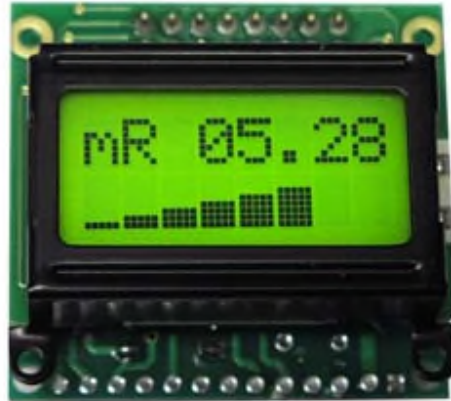
Figure 15.10 - Close up of the Analog Radiation Edge Meter.
