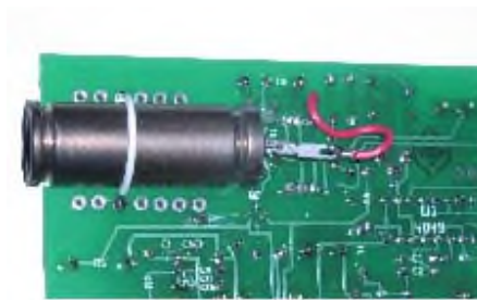
Figure 15.7 - Detail showing GMT-01 tube secured on PCB
