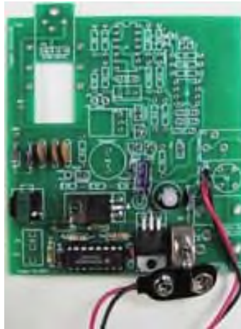
Figure 15.4. Completed HV section of the circuit
