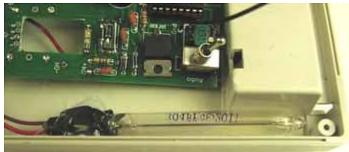
Figure 15.6. GMT-02 Geiger Mueller Tube in Case
