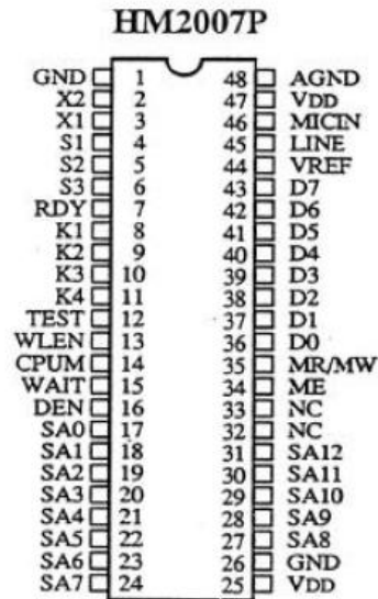
Figure 12: HM2007 Pin Layout [10]
