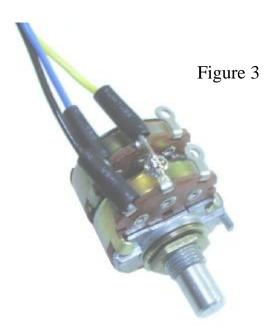
Wire the double ganged potentiometer as shown in figure 3. Next solder the opposite ends of the wires to the printed circuit board, in the box labeled "POT". The center wire of the potentiometer is soldered into the center pad on the labeled box. The two end wires are soldered into the pads on either side of the center position.
