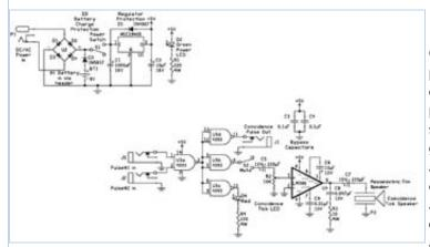
Our coincidence circuit has two pulse inputs and one pulse output. When two pulses are presented on the inputs at the same time, an output pulse is generated. Coincidence circuits are used in nuclear physics experiments. Two examples of applications for a coincidence circuit is a gamma ray telescope and a quantum entanglement
