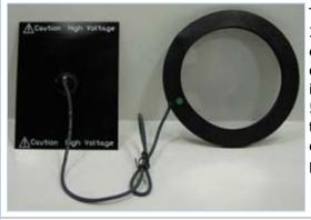
To take Kirlian photographs using a standard 35mm film camera, digital camera or video camera, requires the use of a transparent discharge plate. A transparent discharge plate is constructed from three main components; a 5.5" diameter piece of glass that has a transparent conductive coating (typically tin oxide) on one side, see parts list, a transfer plate and connecting HV wire.
