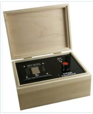
This detector uses a 8000 volt negatively-charged electrode and thin copper wires connected to ground strung approximately 0.1" above the electrode, to detect alpha particles.
