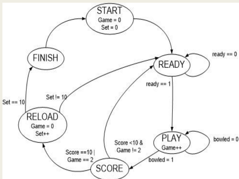
Figure 11: Finite State Machine for Virtual Bowling Application
